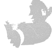
Fig. 17 3D shape reconstruction result using single grid pattern
